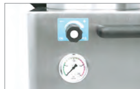
Speed control & pressure gauge
