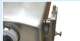
Interlock for carriage disassembly
