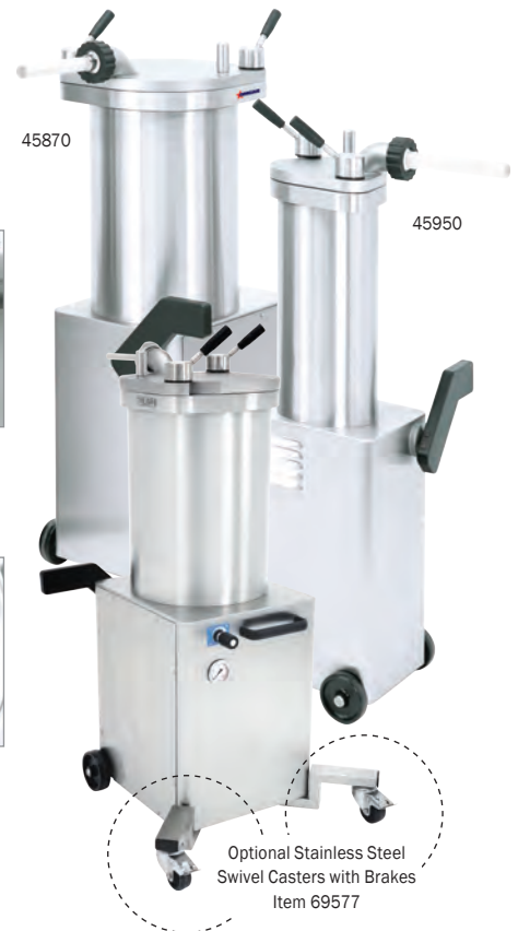
Fully s/s barrel bottom with water draining outlet. Simple cleaning.
