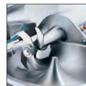
Standard removable 6 and 3-knife head
