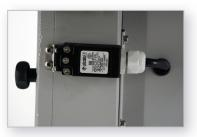
The micro-switch acts as a saftey feature and turns off the machine preventing injuries.
