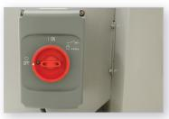
To switch machine on, turn the knob rotation clockwise to the on position. To switch the machine off, turn the knob rotation counterclockwise towards the off position.
