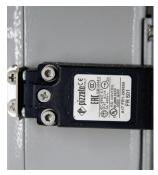
The micro-switch acts as a saftey feature and turns off the machine preventing injuries.
