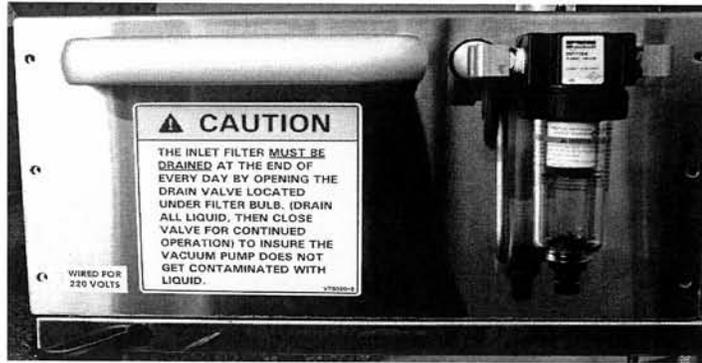
**DAILY:** Drain all moisture from the filter enclosure. Turn the drain knob counter clockwise to drain.
