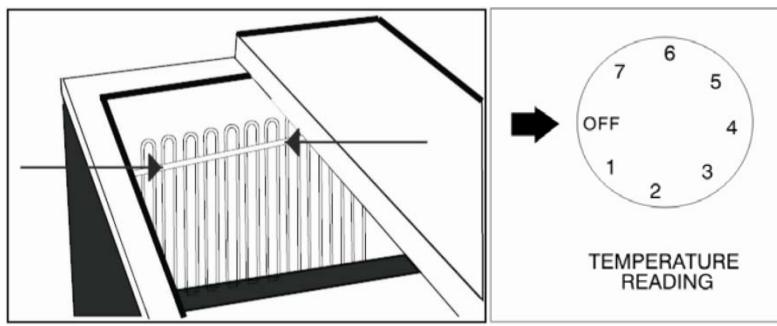
Setting the temperature control to the coldest setting may cause the evaporator coil to freeze and ice up. This will eventually result in a warmer cabinet temperature.
