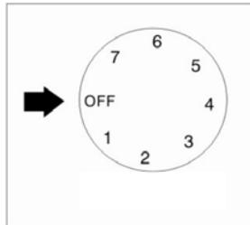
OFF: shut the compressor off.
