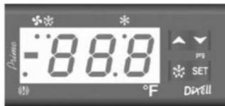
**SET:** to display target set point; in programming mode it elects a parameter or confirm an operation.
