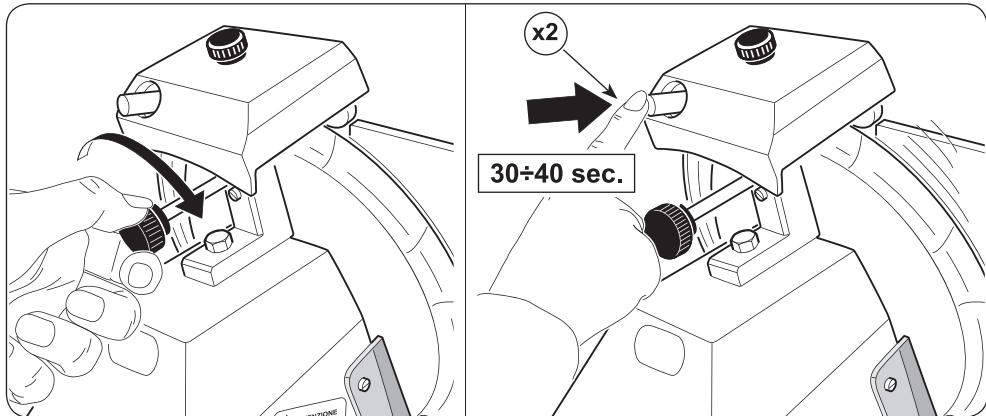
5. Ascertained the formation of the burr, trigger the switch again (1) for 3/4 seconds pressing the little buttons at the same time (x2 and x3).
