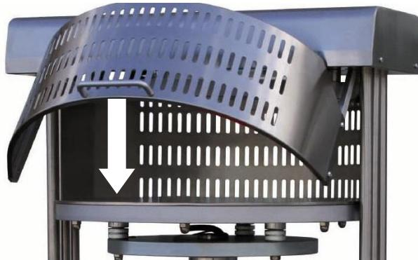
If the first start the bottom plate is not lifted completely, but rises only about 2 cm, the phase sequence is not correct. Reverse 2 phases on the power plug.
