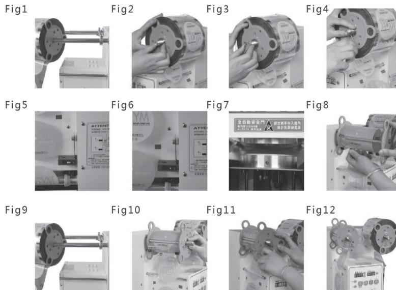
Please note the relative positions between the membrane and all the 6 guide pins.
