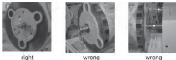
2. The membrane is not installed in the U-type slot of the electrical eye.
