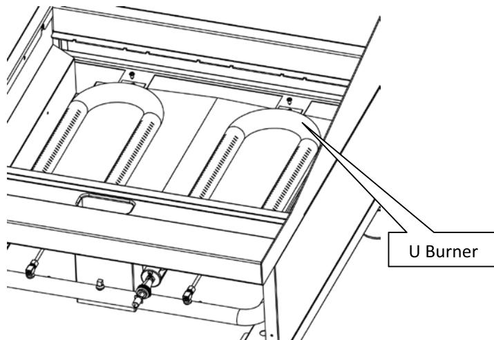
6. Remove the Orifice and Replace it. Use a 1/2" spanner. See the list of Orifice numbers for the appropriate gas type.
