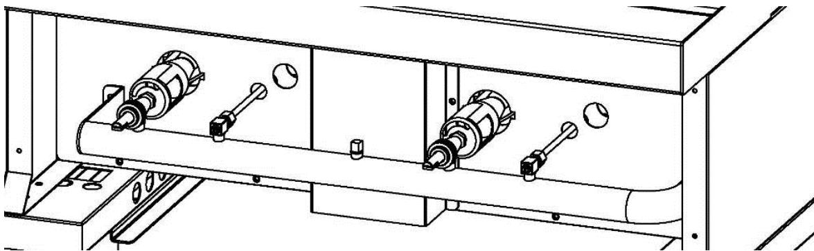
4. Remove the screws for U Burners.
