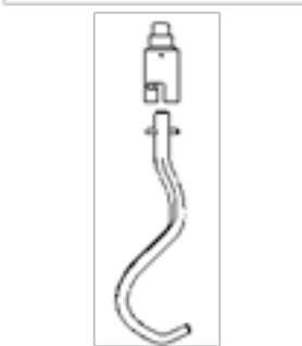
To attach the agitator (i.e., beater, hook, whip) to the mixer, slide the agitator slowly upwards onto the mixer shaft fitting the shaft pin through the slot in the agitator, rotate the agitator 45 degree clockwise to secure it onto the mixer shaft, rotate the agitator 45 degree counterclockwise to remove the agitator.
