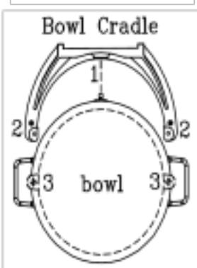
Lift the bowl and slowly position the locking pin into the hole 1 in the cradle, lower the bowl (hole 3 on the bowl) onto the pins located on either of the bowl cradle(hole 2 in the cradle), secure the bowl by pulling each bowl clamp.
