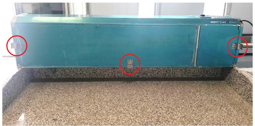
2. Put the topping rail unit on the granite top of the pizza prep table, and the brackets should be placed as following pictures.
