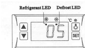
It is a mini-sized and integrated intelligent controller and applicable to the compressor of 1 HP.
