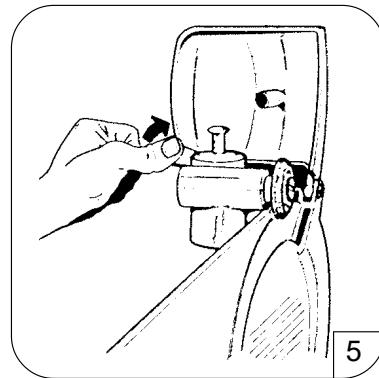
Replace the sharpener to normal horizontal position, by lifting the pin (item (7) and close the cover fig. 6. The grinding stone (item (6), fitted on its pin, can be easily removed, by just drawing it fig. 7. To get a nice sharpening, the grinding stone must be clean and free of grease. The sharpening time depends on the wear of the knife. To get a good result the time needed is 10 to 15 seconds. A longer sharpening reduce the duration of
